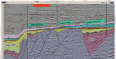
Figure 5a: Interpreted Seismic Profile (from Analyst Presentation Lundin, Norway, press release, 2 December 2010). Mesozoic-Palaeozoic sediments draped on weathered and fractured basement.
